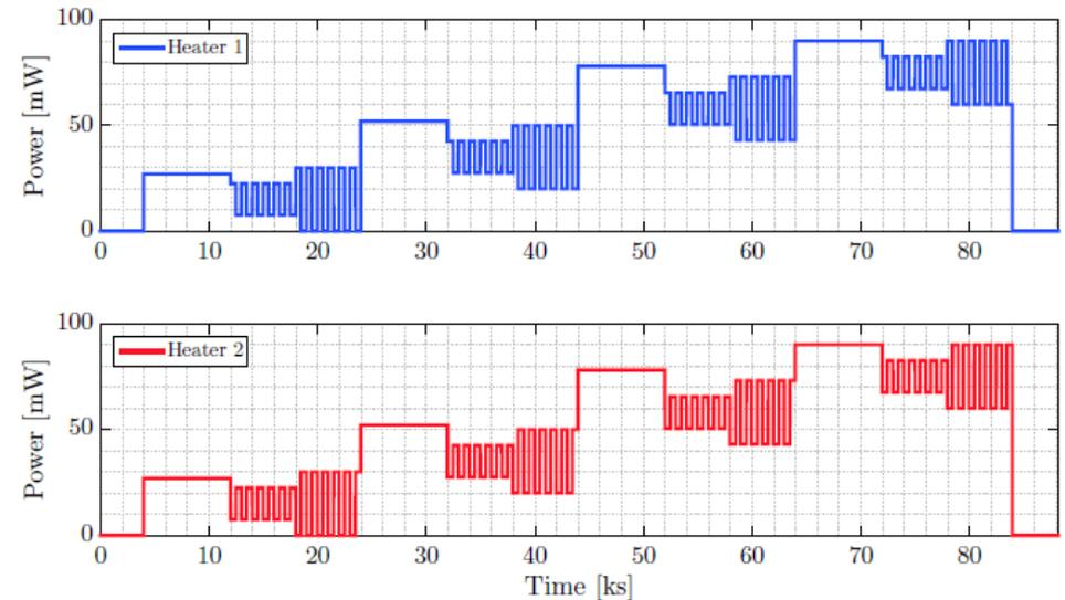
Signal proposed for heaters H1 and H2. As observed, the same modulation pattern is repeated with different DC levels and pre-heating steps.
