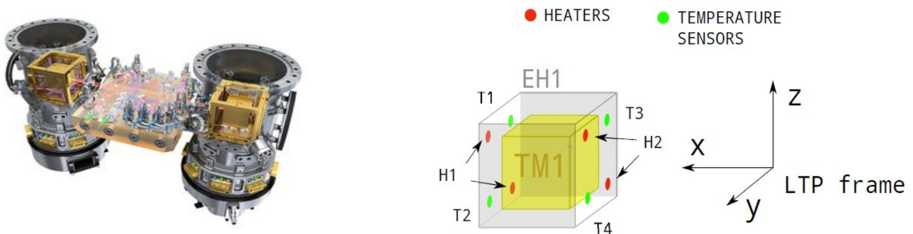
The Electrode Housing experiment aims to estimate the thermal couplings between temperature gradients in the Electrode Housing and direct forces on the Test Masses.
