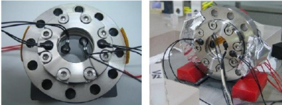
The OW (left), with the plane-parallel plate inside the Titanium flange, heaters on the lateral surface of the latter (pale brown foils) and two pairs of NTC temperature sensors (black beads with wires). On the right, mounting of the OW on rails for measurements. Note heaters are covered with aluminium foils: This is to prevent undesired heating of other components by heaters' emission of thermal radiation.
