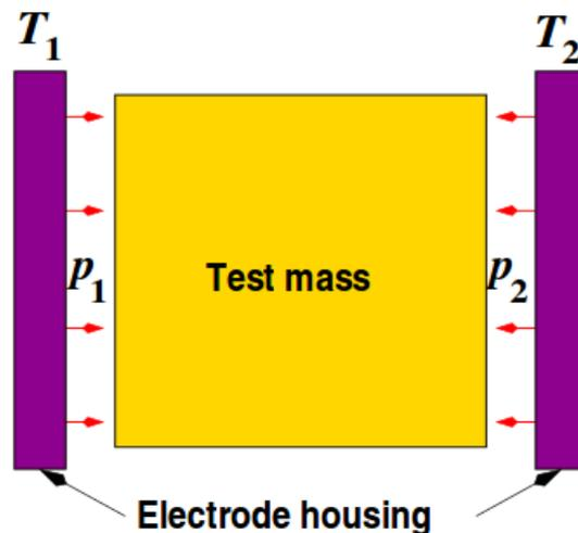
$$F_{RP} = \frac{8}{3} \frac{\sigma}{c} k_{RP} A_{TM} T_0^3 \Delta T$$
