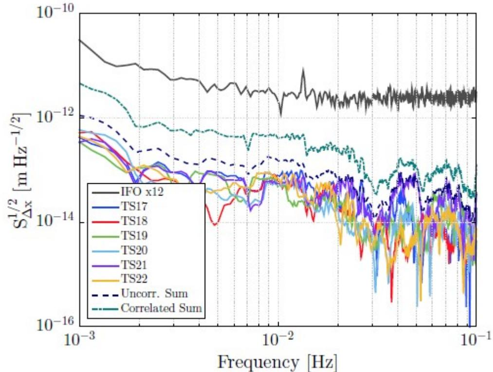
Noise projection of thermo-elastic induced phase noise on the  $x_{12}$ . The contribution from each suspension strut is shown together with the uncorrelated sum of all.
