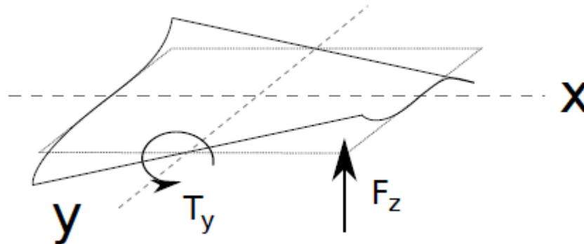
Schematic of the torsion mechanism on  $y$  produced by the vertical component of the force exerted by a heated strut. The case of the image would correspond to a lower strut heater activation such H11 or H14.
