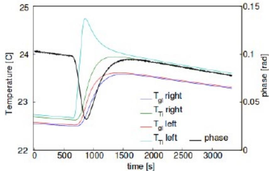
Phase (black curve) and various temperature sensors' responses (coloured curves) to a 2 Watt heat pulse applied during 100 seconds.
