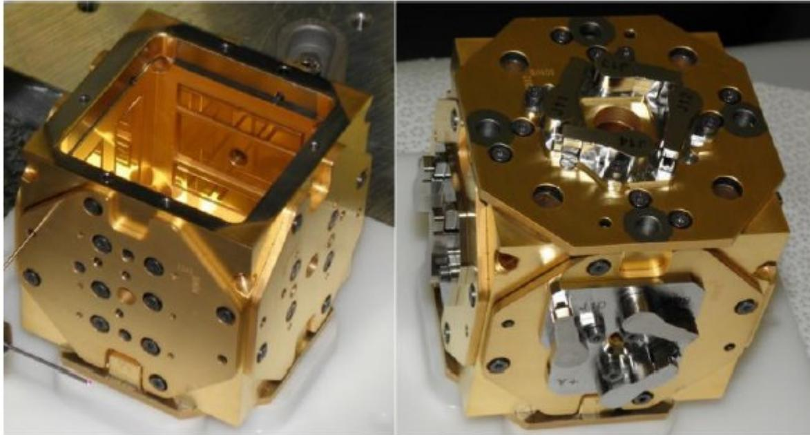
Flight model Electrode Housing.
