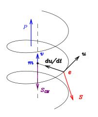
Figure 1. Model of a free Dirac particle, with two separate centers, showing the precession of the CC spin S and the conserved CM spin  $S_{CM}$ . The CC moves along a helix at the speed of light. The CC spin is always orthogonal to the velocity and acceleration of the charge and precesses around p. The separation between CC and CM is  $\hbar/2mc$ , half Compton's wavelength, and the frequency of this internal motion, in the CM frame, is  $2mc^2/h$ . It is described in [2].
